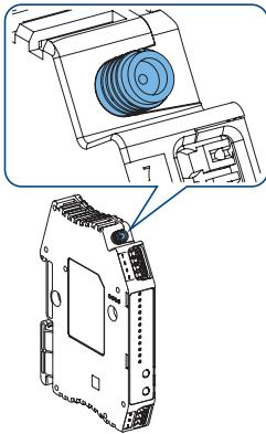
**SMA coaxial connector input:**
