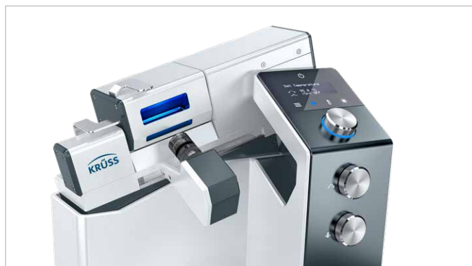
SDT with tilted measuring unit
