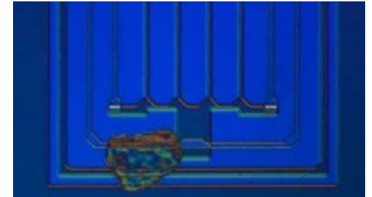
晶圆残留物：反射光、C-DIC；物镜：EC Epiplan-APOCHROMAT 50x/0.95
