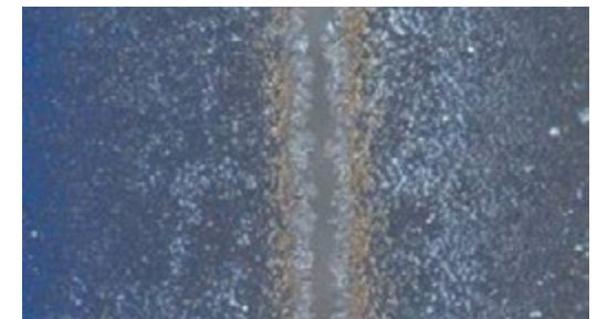
绝缘刻槽：单晶硅太阳能电池上激光刻蚀的绝缘刻槽；物镜：EC Epiplan-APOCHROMAT 20x/0.60
