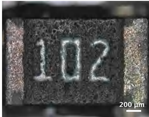
Electronic device SMD resistor: Document the quality of printing and contact surfaces. EC EPIPLAN 5x/0.13
