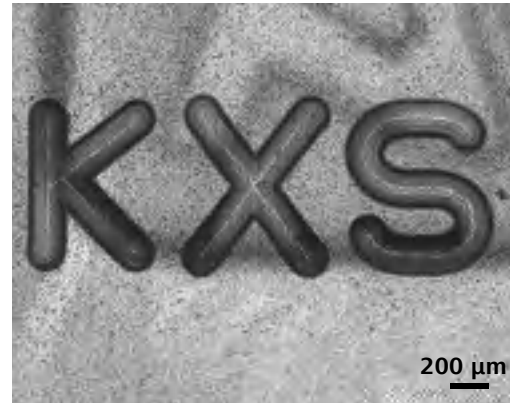
Injection-molded identification letter at transparent plastic part, EC EPIPLAN 5x/0.13
