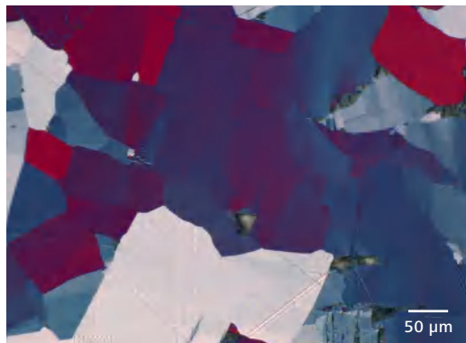
Niccolite, reflected light, polarization contrast with lambda plate, objective: EC Epiplan-NEOFLUAR 20×/0.50 HD DIC
