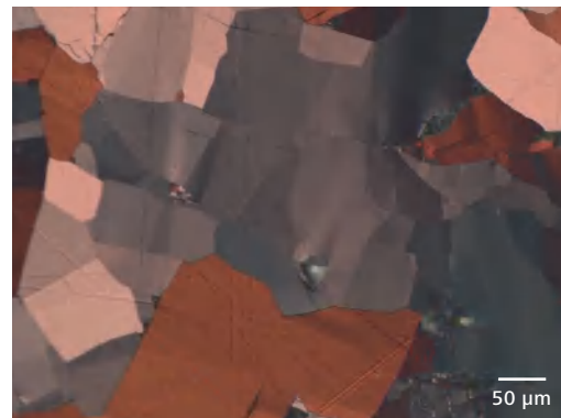
Niccolite, reflected light, polarization contrast with slightly twisted polarizers, objective: EC Epiplan-NEOFLUAR 20×/0.50 HD DIC
