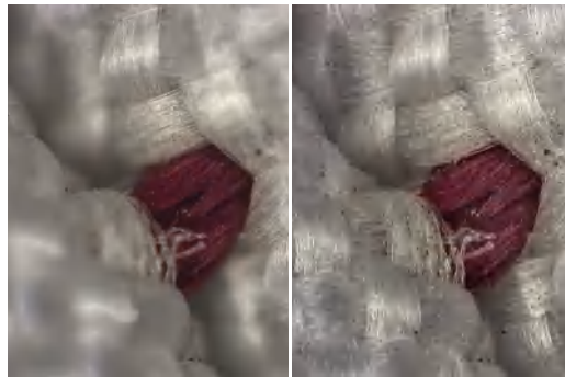
Airbag fabric: without EDF (left); with EDoF (right)
