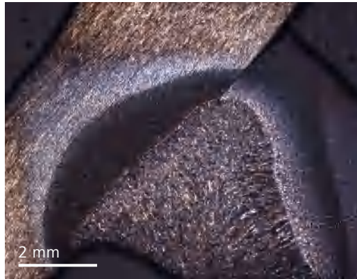
Laser weld, coaxial brightfield illumination, magnification: 35x
