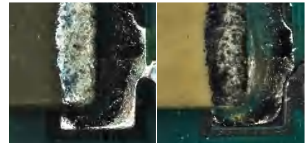
PCB component: without Polarizer Unit (left); with Polarizer Unit (right)
