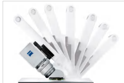
Smartzoom objectives 0.5x, 1.6x and 5x are of sufficiently long working distance to enable tilting of the arm throughout the -45 to +45 degree tilt range, without risk of crashing the edge of the objective into large components, for example PCBs.
