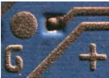
PCB Laterally grazing reflected light Objective: Plan S 1.0x Magnification: 16x*
