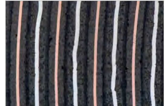
Lithium ionic accumulator, 112x, brightfield
