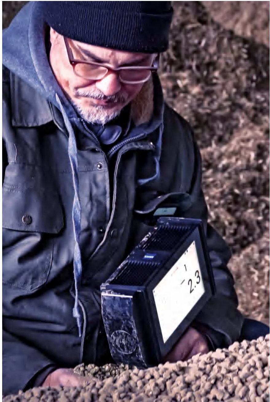
AURA Handheld NIR in the hand of a nutritionist or farmer to measure the quality of the feed for an optimal feed mixture.
