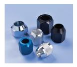
Aluminum retaining nuts are available to hold the Series 141, 160, and 442 mixing nozzles onto adapters, manifolds, and valves and are used when a metal jacket is not required. To attach a mixer to a manifold, press fit the mixer onto the nose of the manifold, slip the retaining nut over the mixer and hand tighten the retaining nut to the manifold.
