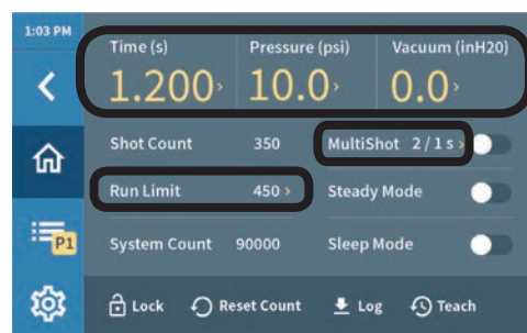
Editable settings on the Home screen: Time, Pressure, Vacuum, Run Limit, and MultiShot
