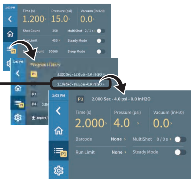
Editing Program 3 (P3) on the Program Details screen while Program 1 (P1) is still the active program
