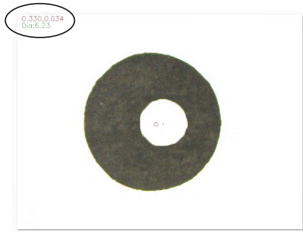
Location of diameter and offset details in the image of a dot that FAILED a positional check
