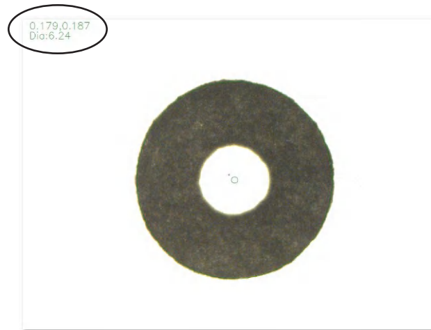
Location of diameter and offset details in the image of a dot that PASSED a positional check
