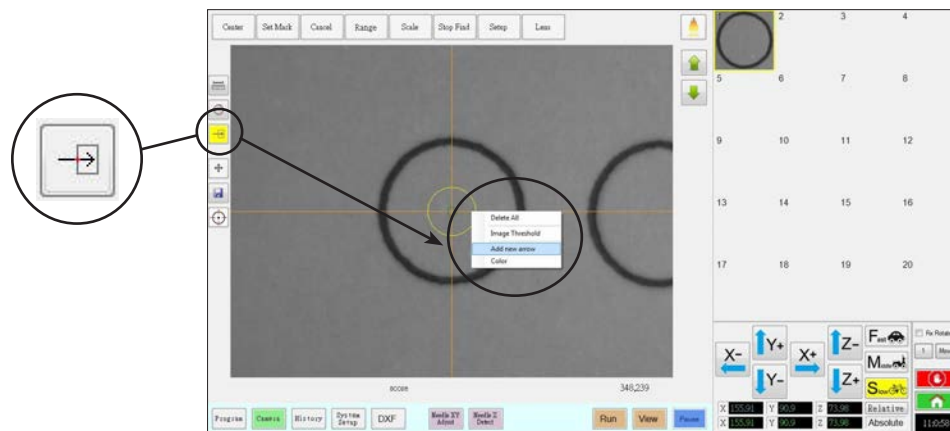
Location of the Arrow icon on the Camera tab (turns yellow when selected) and the resulting menu when you right-click in the Primary View screen
