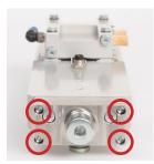
7. • Use the four M4 screws to install the protective housing.
