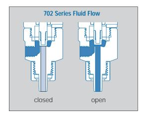
The primary control of deposit size is the valve open time.
