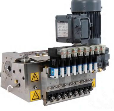
The angled manifold reduces air turbulence common in high-speed operations, increases web-routing options, and facilitates elastic threading. An integrated air heater uses a thin-film flow design that enhances heating efficiency to produce consistent spray patterns and reduce power consumption. A uniform thermal profile improves heat distribution and process stability. Dedicated adhesive recirculation paths provide durability and add-on accuracy.
