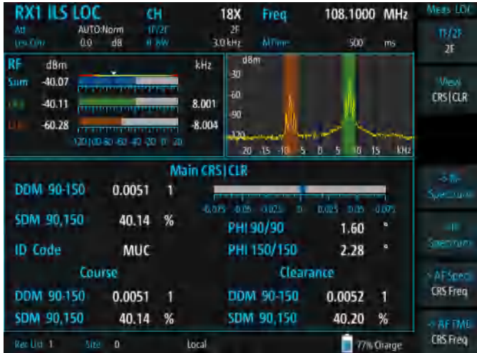
Measurement of a 2F ILS installation
