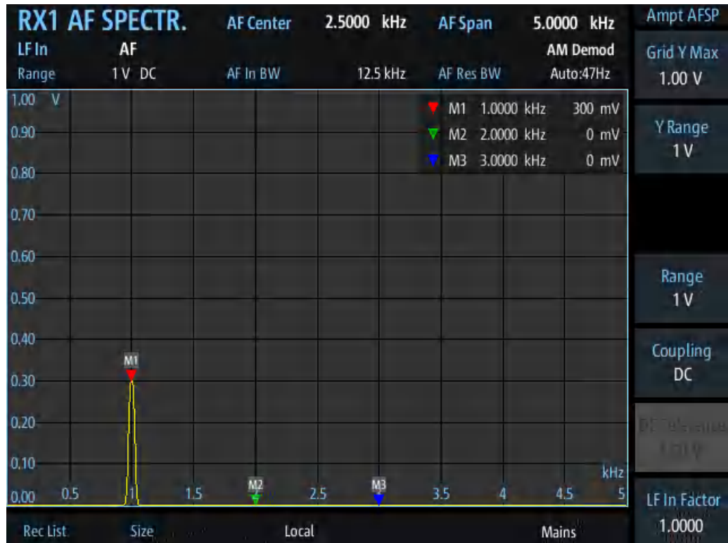
Figure 5-4: AF Spectrum for LF input
