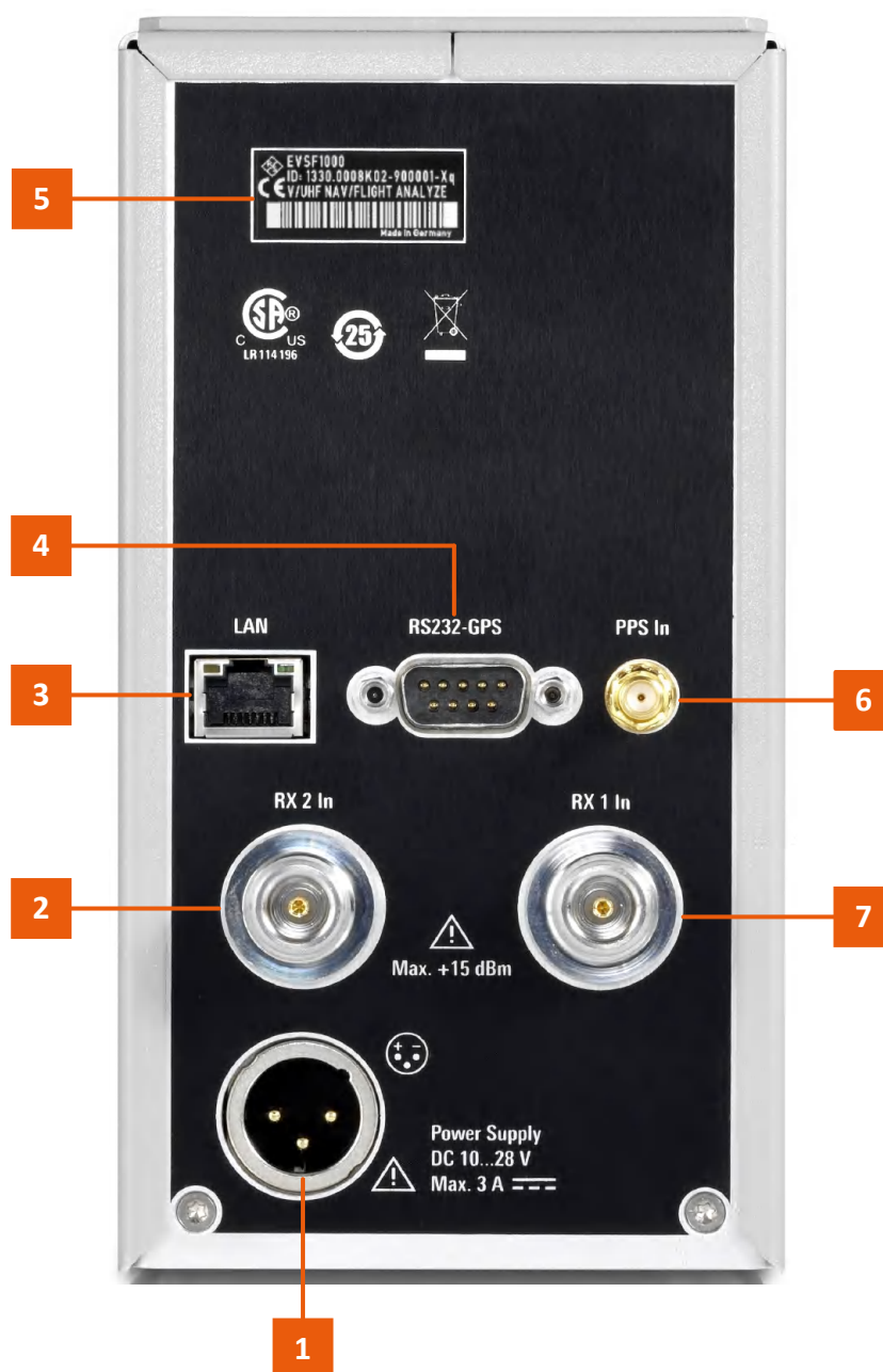
Figure 1-3: R&S EVSF1000 - Rear panel view (basic model, without R&S EVSF1-B4 option)
