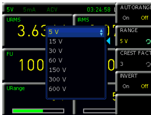
Fig. 5.8: Manual measurement range selection via ACQ menu
