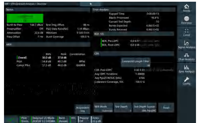
SFD upstream analysis function (with signals from the R&S®SFD) with status display for auxiliary carrier
