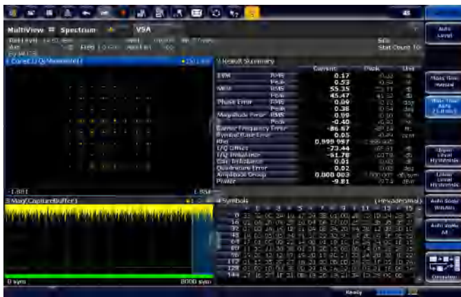
Vector signal analysis of a single carrier 64QAM signal with 5 MHz/s symbol rate.
