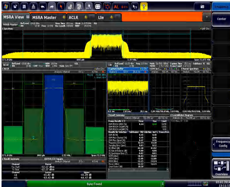
Multiview display of two LTE signals measured on the same I/Q data for interference analysis
