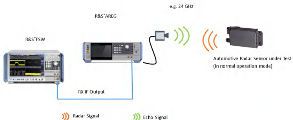
Figure 4-4: Example setup: Analyzing radar signal
