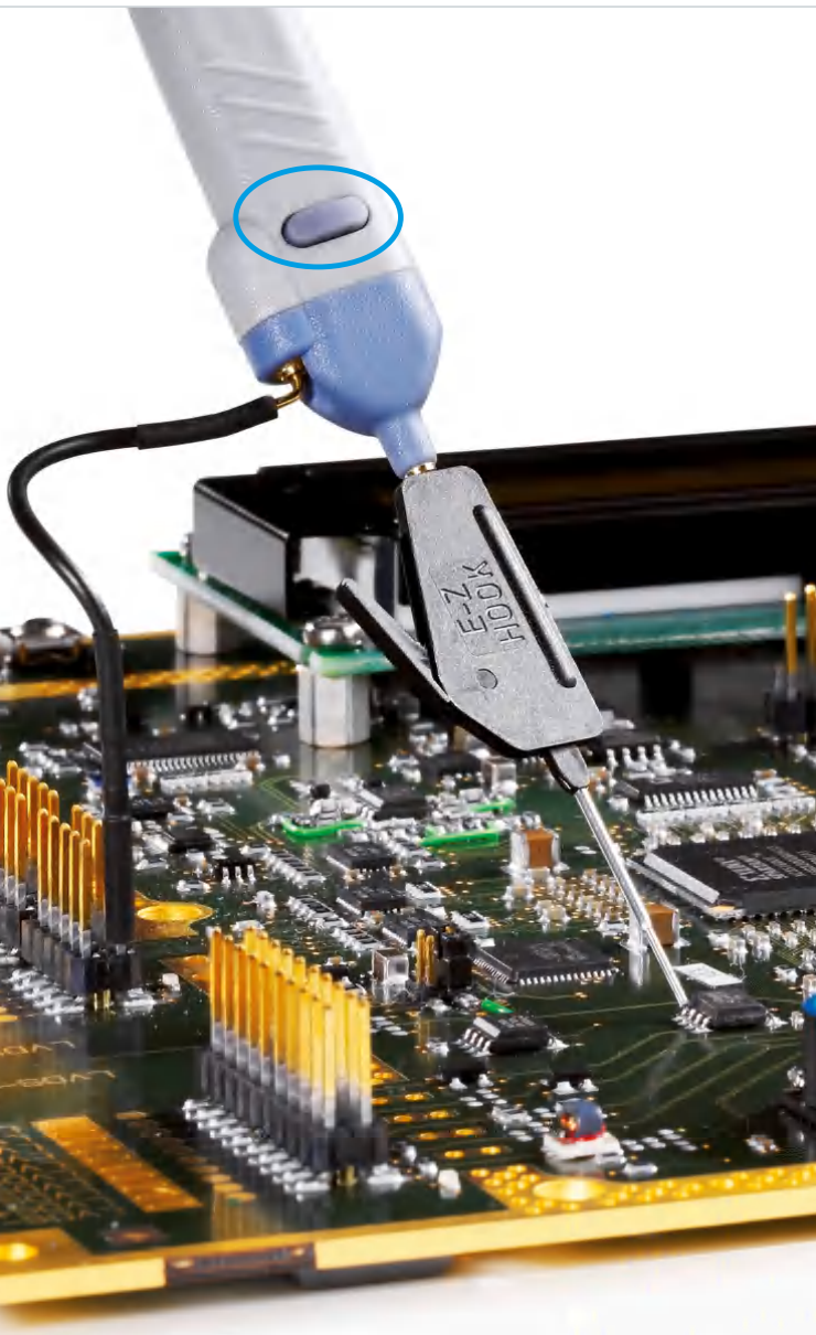
Practical design: micro button for convenient instrument control Diverse probe tips and ground cables are included as standard.
