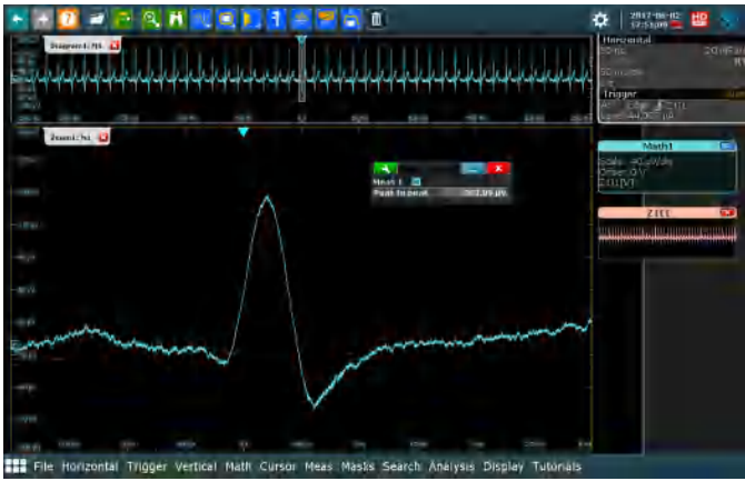
Small signals such as a 200 \mu\text{V} cardiac pulse can easily be measured.
