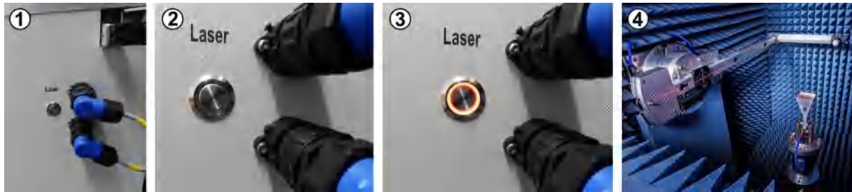
Figure 4-9: Switching on the alignment lasers
