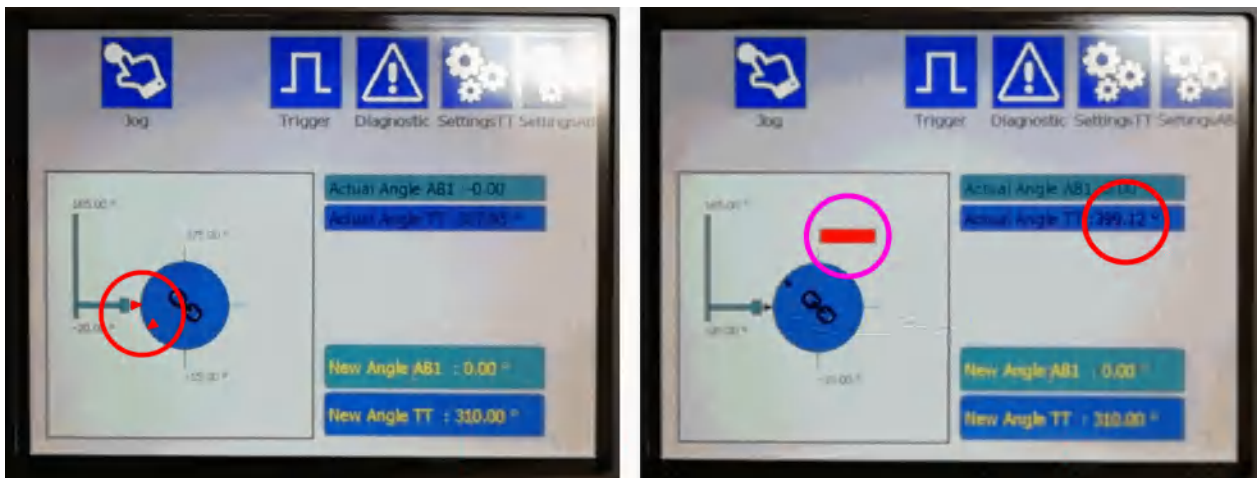
Figure 7-11: During referencing, ignore the red arrows (left) and turntable angles outside of the range from -15° to +375° (right)
