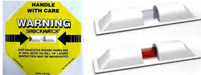
Figure 6-1: Shock indicator, OK if colorless, broken if red
