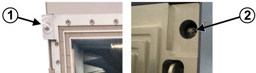
Figure 4-6: Upper interlock key for the door locking mechanism
