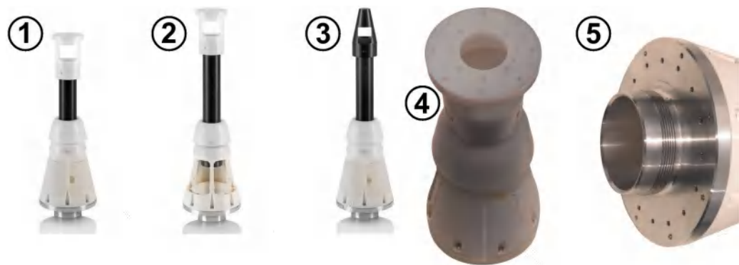
Figure 7-6: Examples of telescopic DUT holder configurations with various adapters
