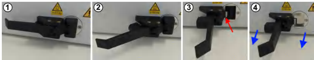
Figure 7-4: Manual opening procedure
