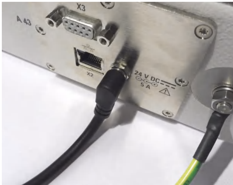
Figure 7-1: 24 V DC power supply connector [X1] (center)
