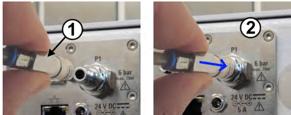
Figure 6-5: Connecting the compressed-air supply
