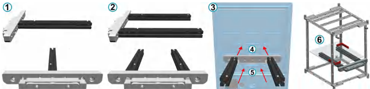
Figure 7-9: R&S CMQ-B712A "Drawer Support 1" option, order no. 1537.6310.02, with door adapter (gray) and holder struts (black)
