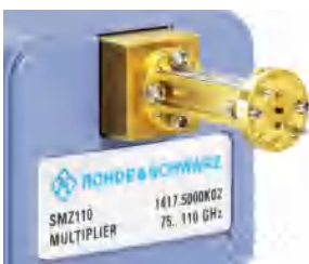
Figure 4-1: Front of an R&S SMZ at the example of the R&S SMZ110 without attenuator
