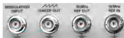
Fig. 7.3: Signal inputs and outputs including modulation input
