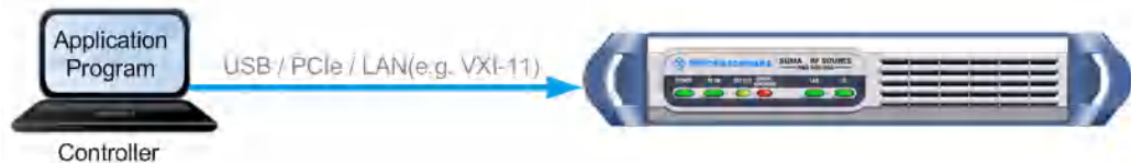
Figure 7-2: Configuration example: remote control from a controller
