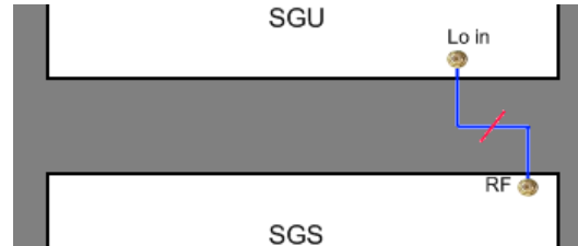
Figure 7-6: A faulty connection between an R&S SGU and an R&S SGS
