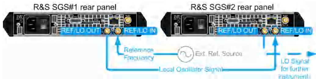
Figure 11-3: Example of a setup: LO coupling
