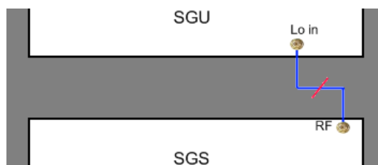
Figure 9-10: A faulty connection between an R&S SGU and an R&S SGS
