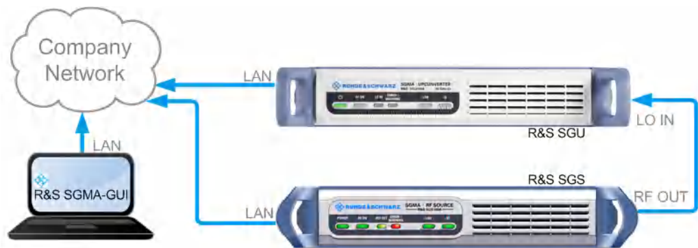
Figure 7-5: Connection of an R&S SGS and an R&S SGU in a company network
