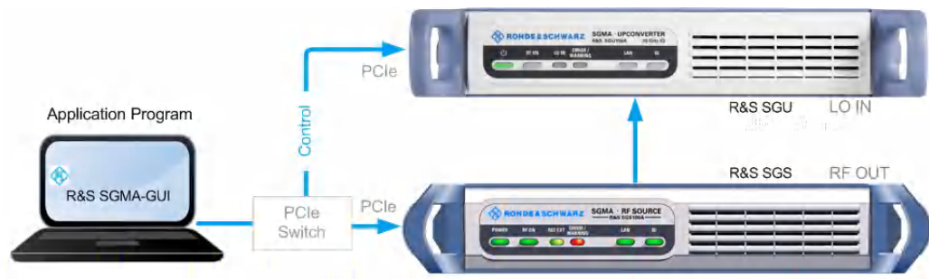
Figure 7-7: Connection of an R&S SGS and an R&S SGU through a PCIe switch
