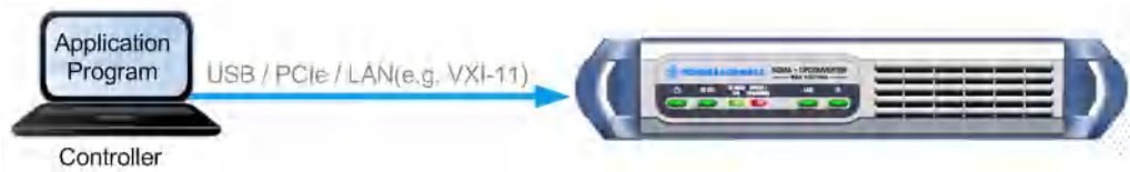
Figure 7-2: Configuration example: remote control from a controller
