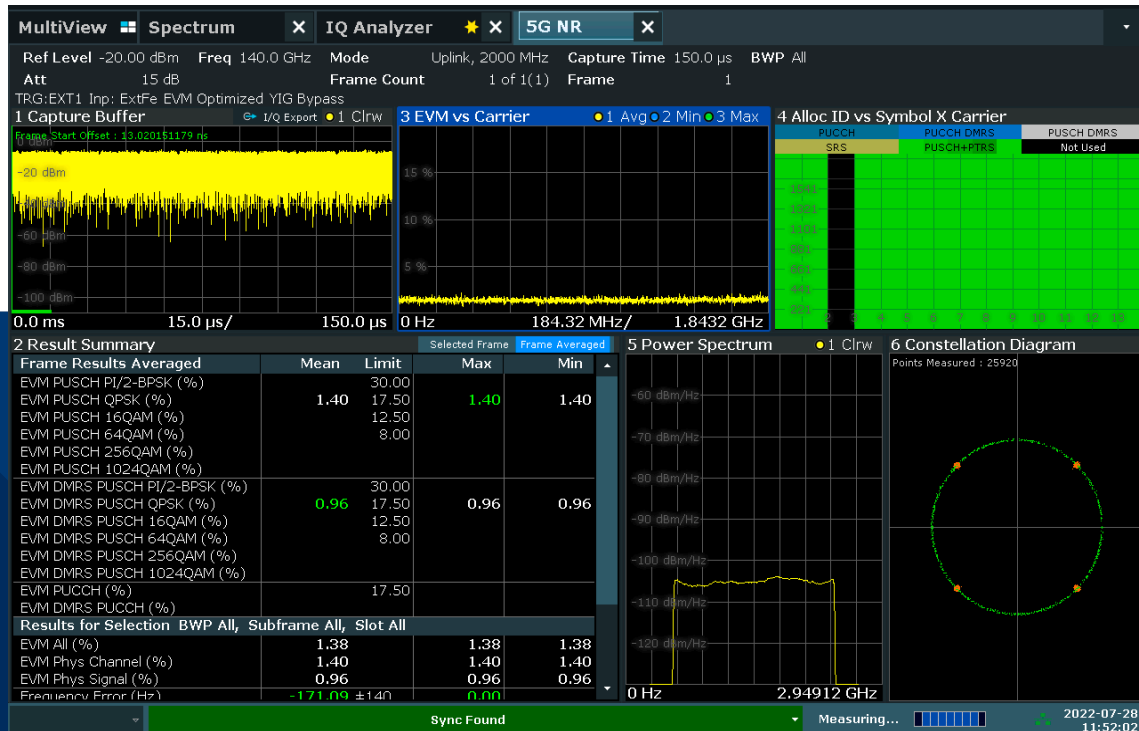
5G NR uplink signal with 2 GHz bandwidth and 148 GHz center frequency.
