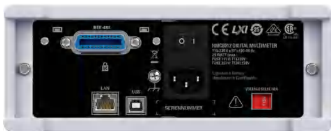
Fig. 1.2: Rear panel of the HMC with voltage selector and connectors
