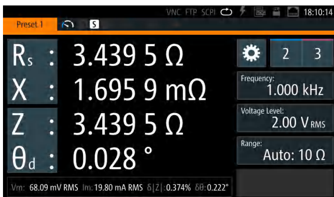
Up to four measurement parameters can be shown on the display at the same time
