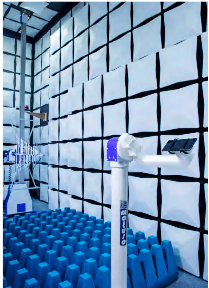
R&S®TS8996 RSE test system covering 2G/3G/4G/5G/Wi-Fi®/Bluetooth®.
