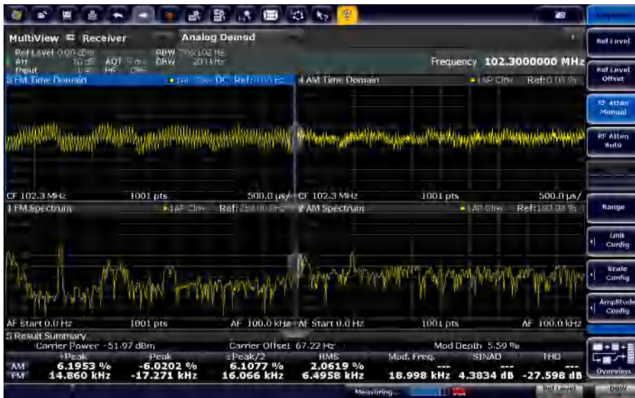
Analog demodulator with multiple result windows
