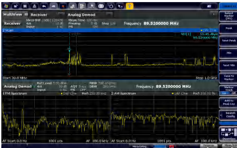
MultiView display: The marker for the previously measured frequency spectrum (top) is coupled with the receive frequency of the analog demodulator (bottom)
