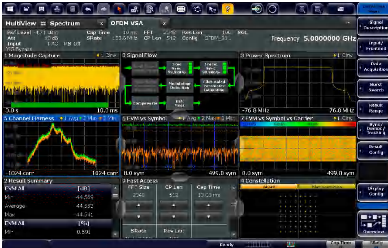
Demodulated OFDM signal with 2048 carriers, 64 QAM, QPSK pilot
