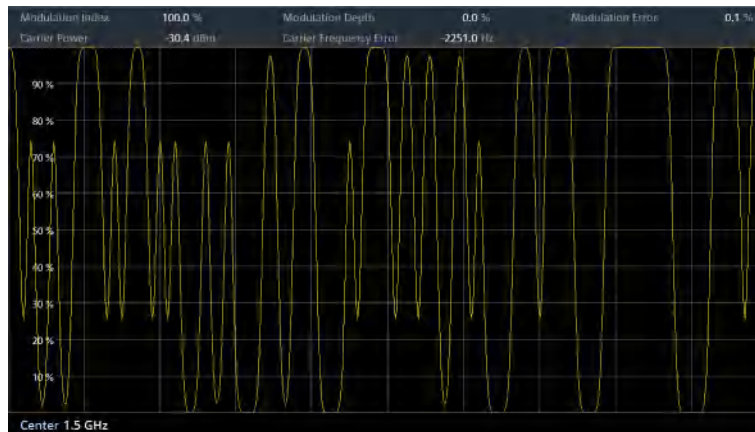
Figure 17-4: Modulation depth of a 2ASK signal
