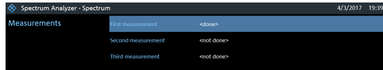
Figure 13-3: Measurement specification shows the measurement sequence
