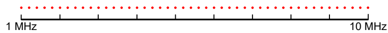
Figure 15-3: Linear x-axis scaling: the distance between the measurement points is equal, e.g. 200 kHz
