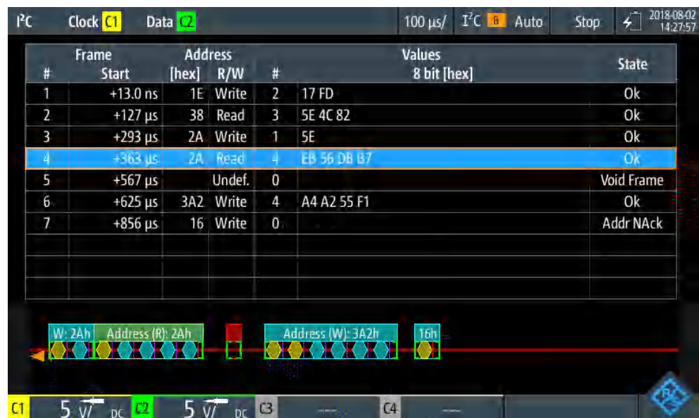
Figure 9-5: Decoded I2C signal with active Track in Table, and reference point set to the left.
