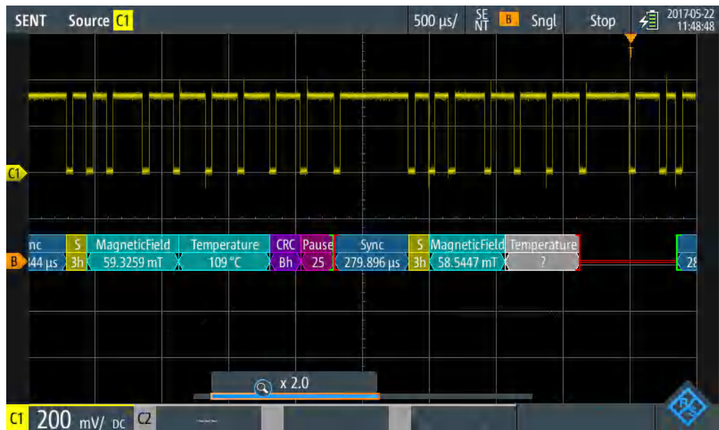
Figure 9-42: SENT decode results with label list translation
