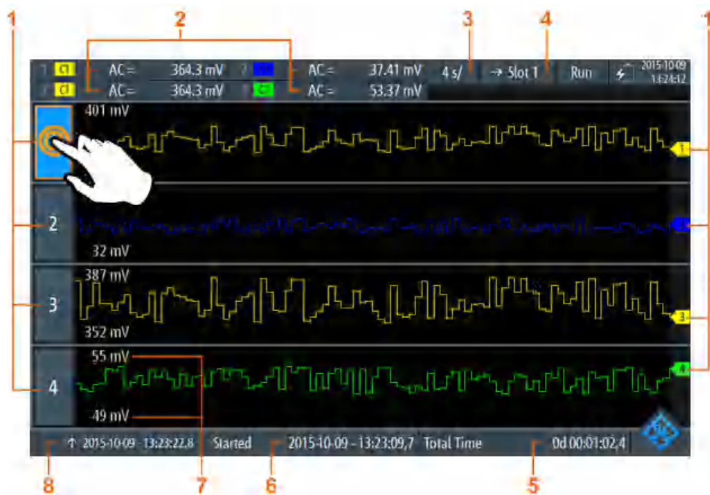
Figure 8-1: Logger display, view of all logged scope measurements
