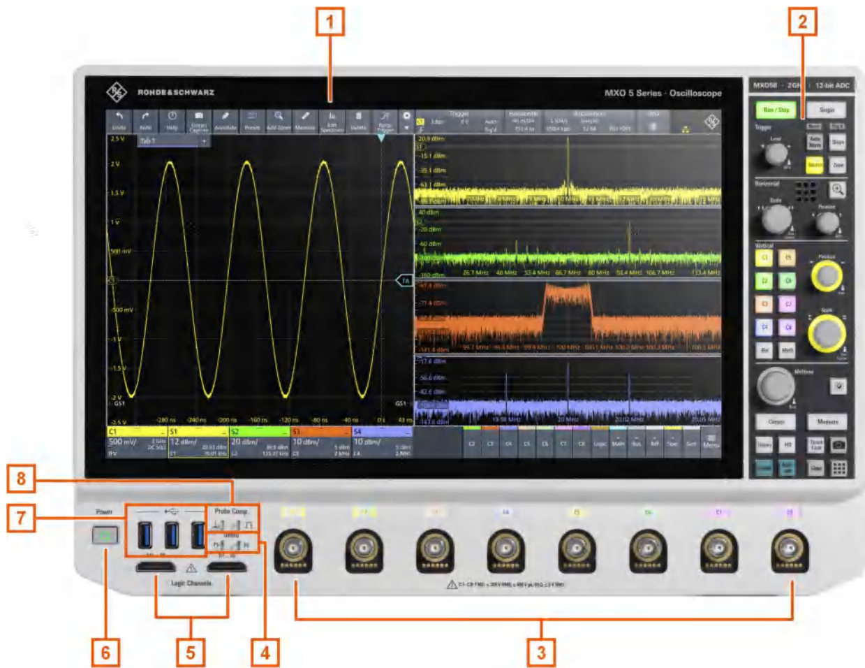
Figure 3-1: Front view of R&S MXO 558, with 8 input channels
