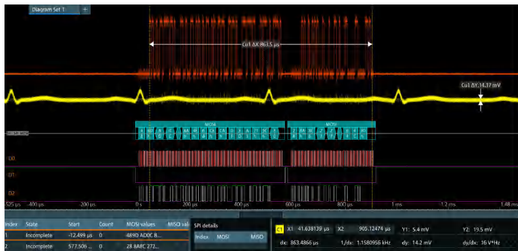
Figure 13-3: Decoded and binary SPI signal
