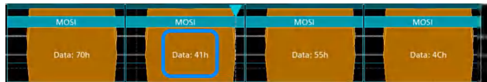
Figure 13-4: Trigger on Type= MOSI, Data pattern = 41
