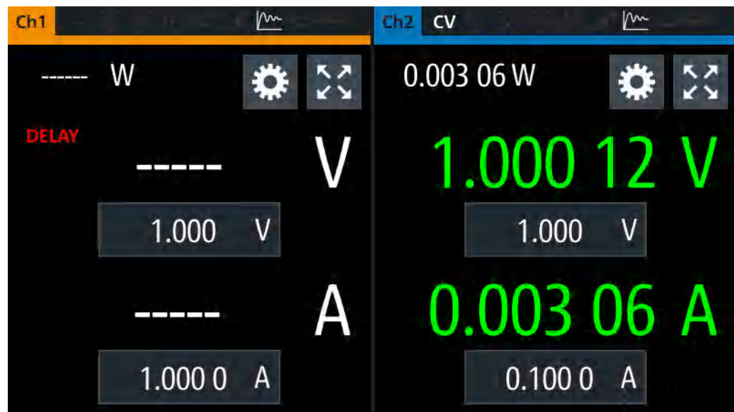
Figure 6-10: Delay text at channel display area
