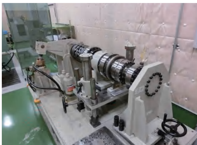
Durability testing with continuous load testing system
