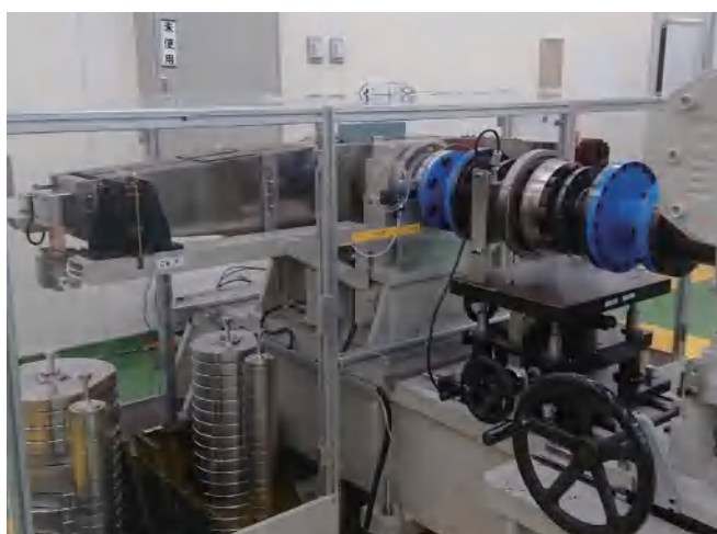
Calibration with a high-precision torque reference device
