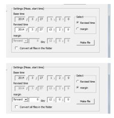
• To convert all measurement data files in the folder in which the specified measurement data file is located, select the [Convert files in folder] checkbox and click [Make file].
