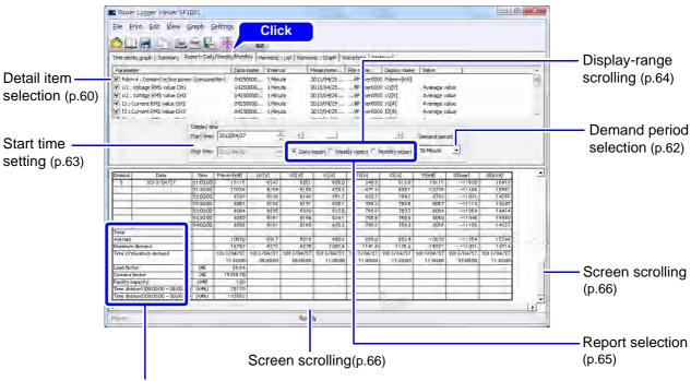
When the **[Pdem+ demand active power]** parameter is selected, the active power demand value (consumption) total, average, maximum demand, maximum demand time, load rate, demand rate, and Facility capacity will be displayed.
