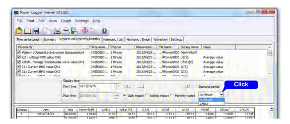
**NOTE** An interval smaller than the measurement interval of the loaded data cannot be set.
