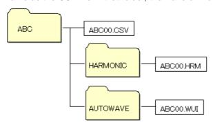
• For Model 3169, if there is a waveform data file that is the same type as the CSV file (extension: WUI), the waveform data file will also be loaded.
