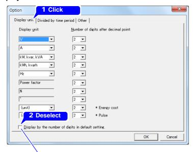
Selecting this checkbox causes data to be displayed using the number of measurement data digits, without regard to the number of decimal places setting.
