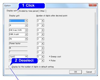
Selecting this checkbox causes data to be displayed using the number of measurement data digits, without regard to the number of decimal places setting.
