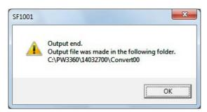
The converted file will be output into a new folder created with the name "ConvertXX" (where XX indicates an automatically allocated value from 00 to 99) in the same folder as the specified measurement data file (.csv).
