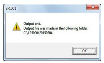
The converted file will be output into a folder with the same name as the LR5000 representative file (.hrp2) located one level lower in the file hierarchy than the original file.
