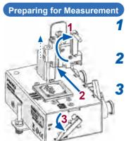
Turn the pusher up/down operation knob in the "up" direction to raise the tip pin.
