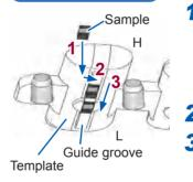
Place the sample on the template using a pair of tweezers.
