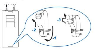
**3** Attach the strap buckle to a compatible instrument and connect it to the clip that you attached to the device with the strap.
