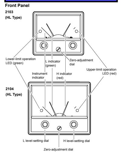
(The H type and the L type have only one operation LED on either side and only one level-setting dial on the right.)
