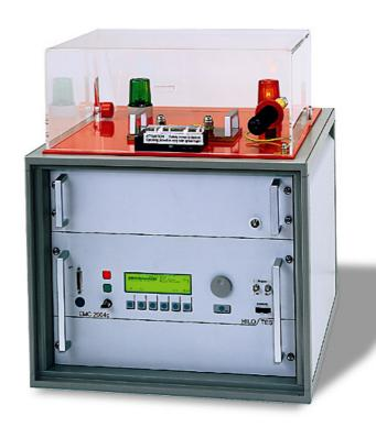
The high-current pulse generator PG 6-2402 is designed for surge current testing of electrical components, over-voltage protectors and electronic circuits acc. to IEC, VDE etc. It generates standard impulse currents with waveform  $8/20\mu s$ . Pulse current output amplitude can be set to 2 - 50 kA.
