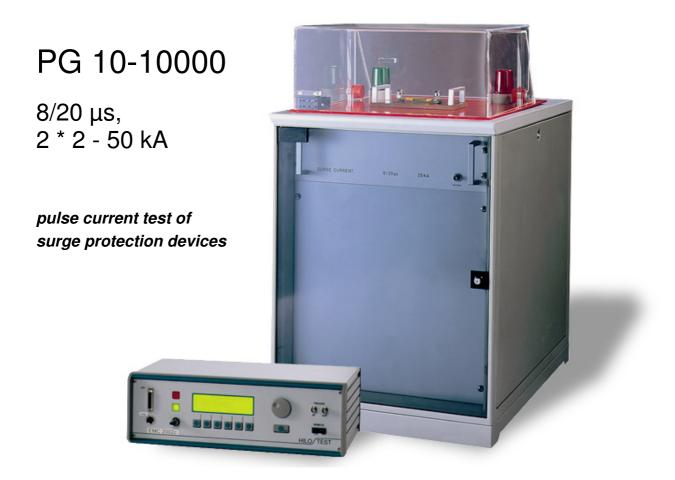
The SURGE TEST GENERATOR PG 10-10000 delivers surge current pulses with the waveform 8/20µs, acc. to IEC 60. It was designed for testing surge protection devices. Moreover the generator can be used for testing two-gap over-voltage protectors. It delivers surge current pulses synchronous at two impulse current outputs, peak value adjustable 0.5 - 50 kA for each output. Positive or negative polarity of output current can be selected.
