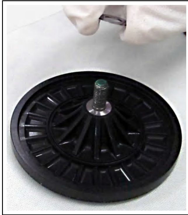
Figure 7-11 Placing original spacers on new diaphragm
