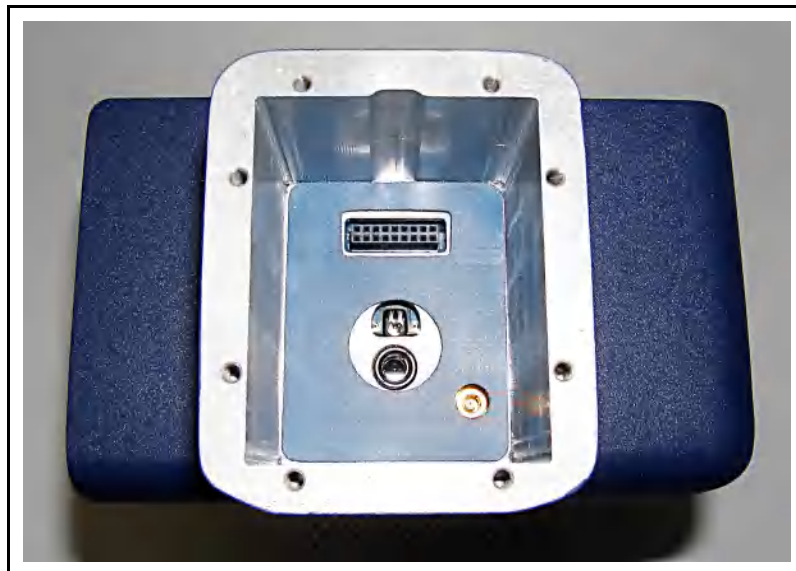
Figure 6-7 Inner Gasket Installed
