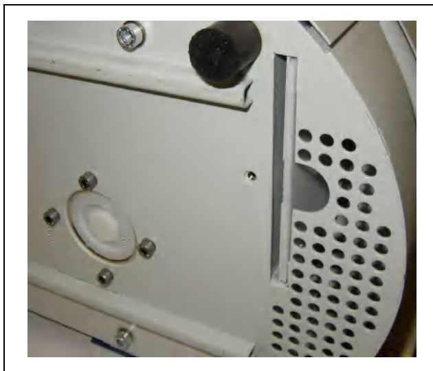
Fig. 8-2 Dismounting of the air filter
