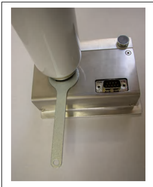
Fig. 8-18 Installing the gas reservoir
