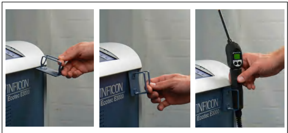
Fig. 1-6 Installation of sniffer line holder
