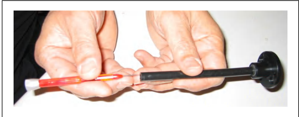
Fig. 8-14 Pushing out the steel capillary
