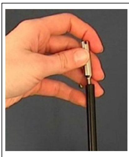
Fig. 1-7 Installing water protection tip
