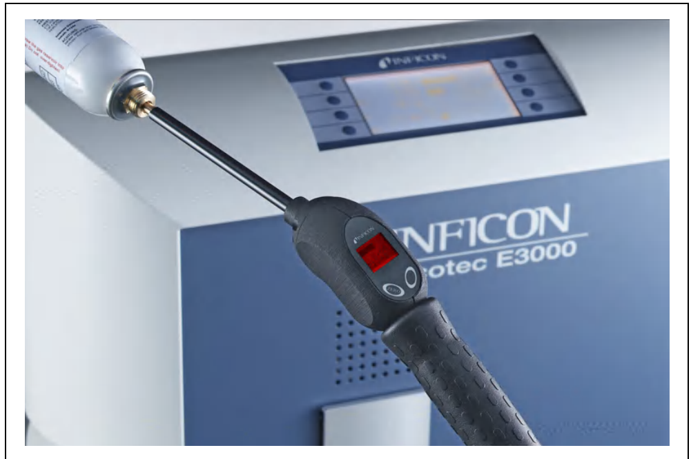
Fig. 3-6 Sniffer display when detecting a leak
