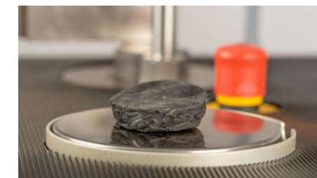
Integrated sample balance with automatic measured value transfer
