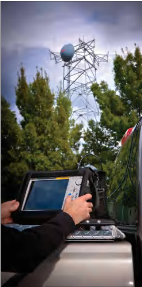
LMR Master testing from a service vehicle
