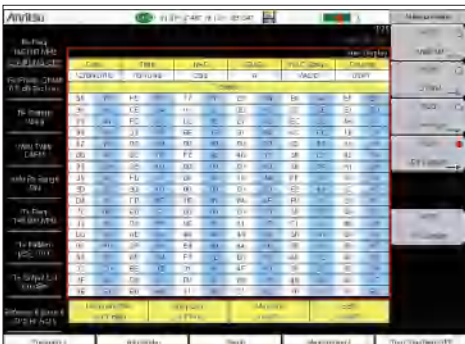
The P25 Bit Capture display displays the uplink traffic and exports this to USB memory.
