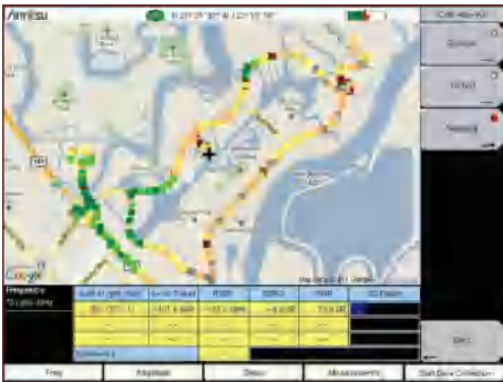
Over-the-Air Measurements – Tx Test By looking at the reference signals of MIMO antennas one can determine if MIMO is working properly. If the delta power is too large, there is an issue.
