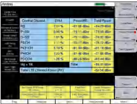
Modulation Quality – Control Channels High values will create larger areas of cell-to-cell interference and create lower data rates near cell edges. Low values affect in-building coverage.
