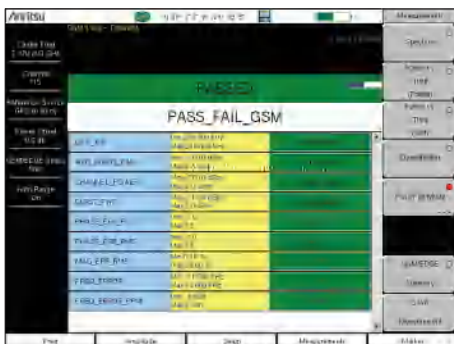
Pass/Fail Test Set up common test limits, or sets of limits, for each instrument. Inconsistent settings between base stations, leads to inconsistent network behavior.
