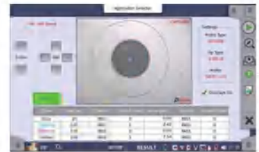
MT1000A screen displays details of the fiber tip core, cladding, adhesive and contact, with automatic Pass/Fail result judgement.
